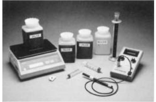
FIGURE B.3(d) Sampling Equipment and Samples for FFFP Concentration Test.
