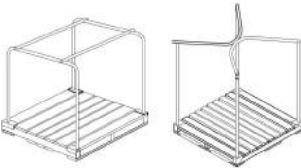
FIGURE A.3.3.191(b) Typical Palletized Portable Tire Rack Units.
