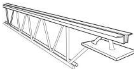
FIGURE A.3.3.43.2(b) Open-Web Bar Joist Construction.
