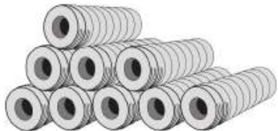
FIGURE A.3.3.191(f) On-Floor Storage; On-Tread, Normally Banded.
