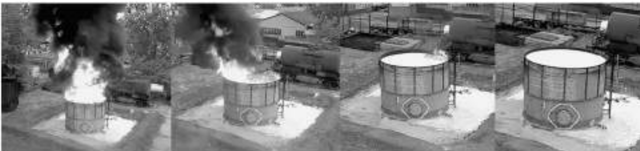
FIGURE H.3.2(c) Extinguishing Sequence, FFF, Subsurface Injection.
