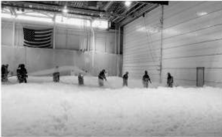
FIGURE A.7.6.2.3(c) Firefighters Sweeping 6 ft (1.8 m) Wands in a 180-Degree Motion Searching for Anything Hidden Beneath the Foam.
